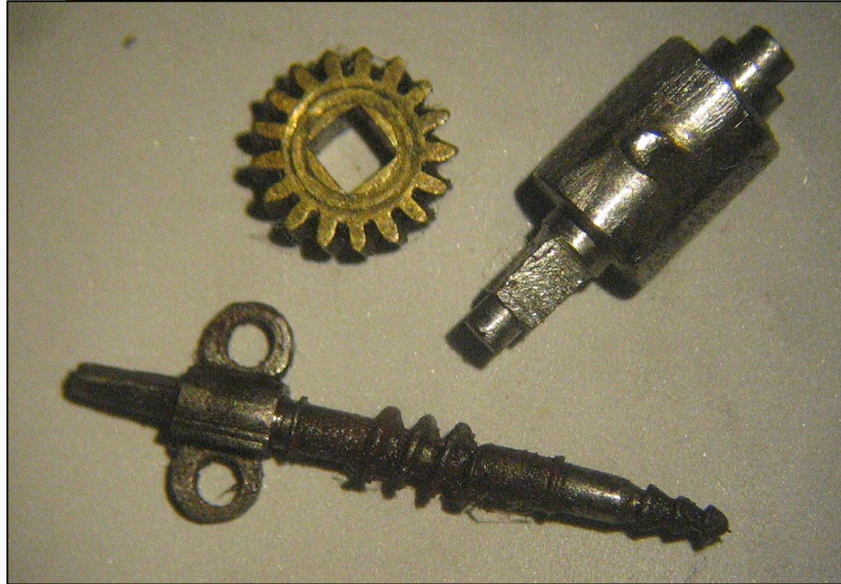
Mainspring pre-tensioning mechanism Intricately hand made on "turns" lathe
